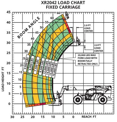
LOAD RATINGS SHOWN ARE FOR VEHICLES EQUIPPED WITH FOAM FILLED TIRES ONLY. 10,000 LBS AT 24 IN MIN CAPACITY FORK (20,000 LBS PAIR).
