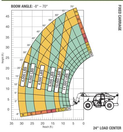
No operation above 40° boom angle with rear axle unlocked. Load ratings shown are for vehicles equipped with foam-filled or solid tires. Load includes weight of any rigging. 5,500 lbs. at 24" minimum capacity/fork (11,000 lbs./pair).
