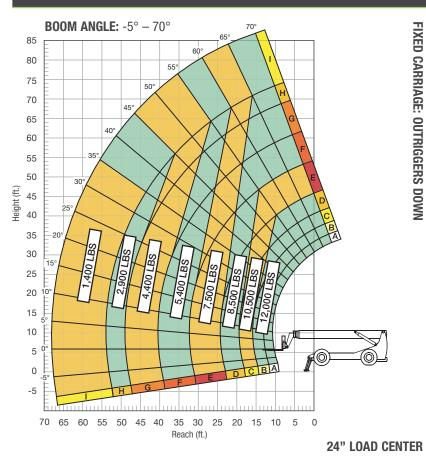
Rear axle must be locked and outriggers firmly against ground. Load ratings shown are for vehicles equipped with foam-filled tires only. 6,000 lbs. at 24" minimum capacity/fork (12,000 lbs./pair).
