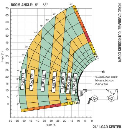
Rear axle must be locked and outriggers firmly against ground. Load ratings shown are for vehicles equipped with foam-filled tires only. 7,500 lbs. at 24" minimum capacity/fork (15,000 lbs./pair).
