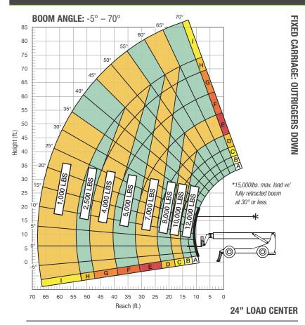
Rear axle must be locked and outriggers firmly against ground. Load ratings shown are for vehicles equipped with foam-filled or solid tires. 7,500 lbs. at 24" minimum capacity/fork (15,000 lbs./pair).
