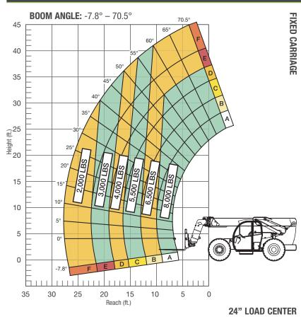
Load ratings shown are for vehicles equipped with foam-filled or solid tires. Load includes weight of any rigging. 4,000 lbs. at 24" minimum capacity/fork (8,000 lbs./pair).
